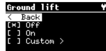
Ground LIFT Custom: allows you to choose which channels to connect to GROUND. Press ENTER to activate ground connection.
