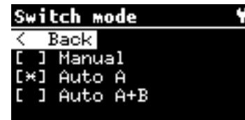
Choose the Switch Mode function to define in which mode the switch between the two machines connected to GO.8 will take place.
