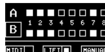
On the GO.8 main screen, you can see in white what audio channels are used and connected. In the line below:
